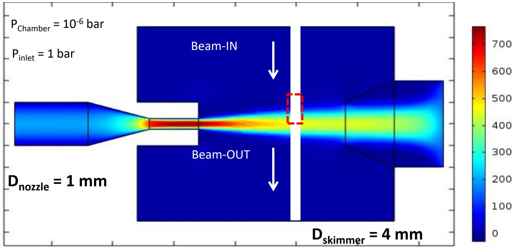
The number of He gas at 10 mm distance from the nozzle expected to be  $\sim 10^{17}/\text{cm}^3$  assuming a 1 mm beam diameter
