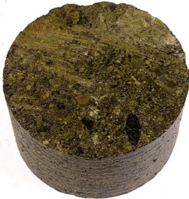
410g drill core f = 74 mm L = 40 mm
