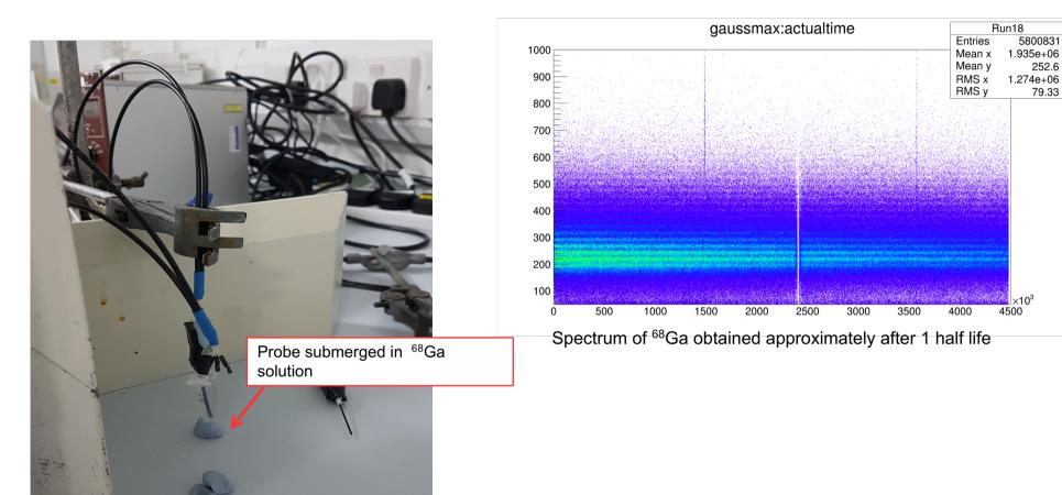
The light output produced by the scintillating fiber was detected by SiPM and converted to electronic signal.
