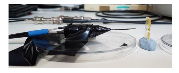
The positron probe consists of bundle of five polystyrene based plastic scintillating fibers (BCF-10 Saint Gobain) 50 mm length painted with reflecting paint and a layer of black paint coupled to SensL 1x1 mm SiPM
